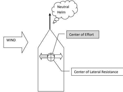
When sailing rudderless in a straight line, we try to keep the <u>COE on top of the CLR</u>.
