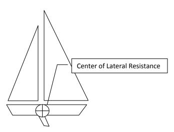
Raising the center board moves the center of lateral resistance back on the boat:
