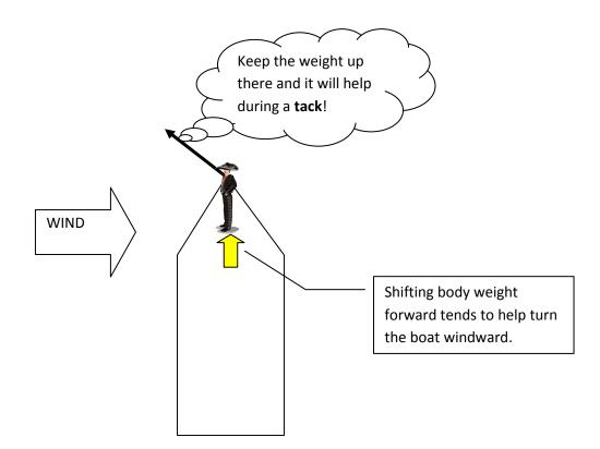
Since these forward/aft weight shifts are smaller, I recommend focusing on lateral weight shifts first while learning rudderless sailing.
